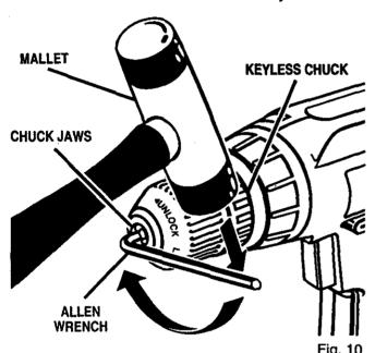
Open chuck jaws and remove allen wrench. Remove the chuck screw by turning it in a clockwise direction. See Figure 11. Note: The screw has left hand threads.
